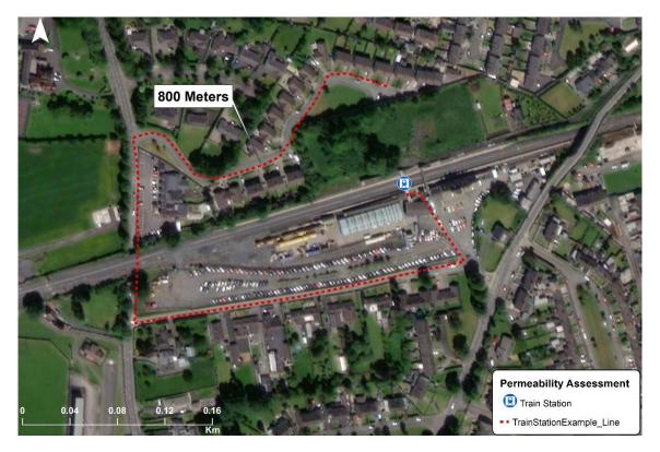
Figure 4.27: Example of Indirect Travel due to Cul-De-Sac Design and Boundary Walls
